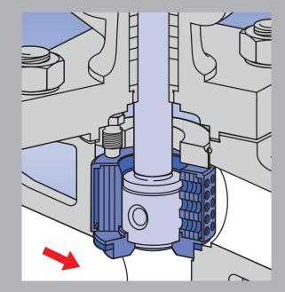
The control edge permits the function of a conventional isolating valve and a control valve to be combined in one unit, and achieves very low leakage rates. Here the valve plug is shown in the closed position.
