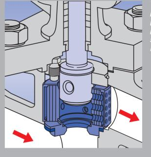
position. Irrespective of the position of the valve plug, the pressure is always reduced in several stages, even for the lower control range.
