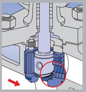
At the beginning of the opening process, the valve plug lifts off the seat but the control edge does not set any orifices free yet. At the moment of opening or closing, the flow velocity at the valve seat is zero, so that wire drawing is excluded.
